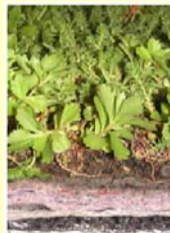
XF301 Sedum Mat (1 1/2") XF159 Water Retention Fleece (1/2") XF108H Drainage Layer (1/2") (not shown: XF112 Root Barrier 20mil LDP)
